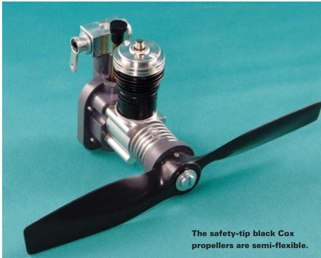
The safety-tip black Cox propellers are semi-flexible.
