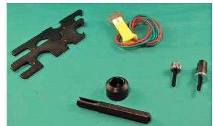
These engines are not difficult to work on, but do require the proper wrenches, which are available from Cox International. Never stick anything into the exhaust ports as the soft steel cylinder is very easy to damage.
